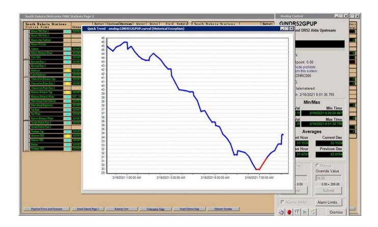
This is an example of pressure trending visible to us via Scada. We were using this type of chart extensively throughout the event.
